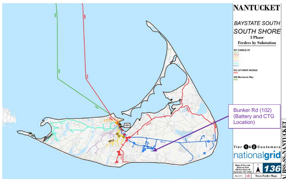
Figure 2.1. Town Feeder Map (13.2 KV) for Nantucket Island, with 46-kV Cables and Battery/CTG Location
