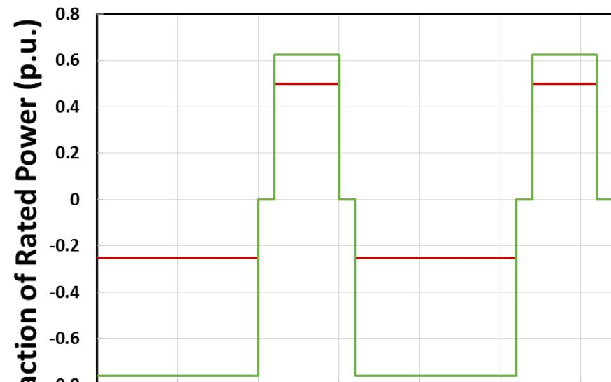
**Figure 3.** Peak shaving with var duty cycle 1; C/2 rate discharge, C/4 rate charge, maximum apparent power 0.8 p.u. (top) E/P = 1, (bottom) E/P = 2. For E/P < 1, the duty cycle looks identical to E/P = 1 once the power is derated to be equal in magnitude to the rated energy.
