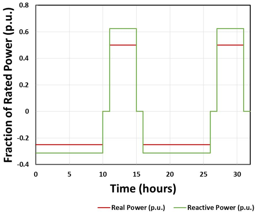
**Figure 4.** Peak shaving with var support duty cycle 2; C/2 rate discharge, C/4 rate charge, maximum apparent power 0.8 p.u. during discharge, power factor during charge set equal to power factor during discharge (top)  $E/P = 1$ , (bottom)  $E/P = 2$ . For  $E/P < 1$ , the duty cycle looks identical to  $E/P = 1$  once the power is derated to be equal in magnitude to the rated energy.
