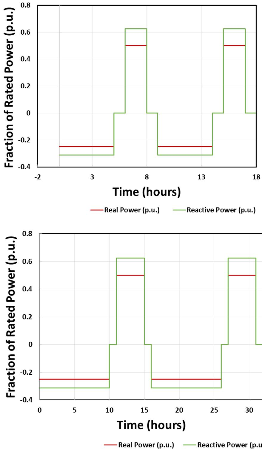
**Figure 4.** Peak shaving with var support duty cycle 2; C/2 rate discharge, C/4 rate charge, maximum apparent power 0.8 p.u. during discharge, power factor during charge set equal to power factor during discharge (top) E/P = 1, (bottom) E/P = 2. For E/P < 1, the duty cycle looks identical to E/P = 1 once the power is derated to be equal in magnitude to the rated energy.
