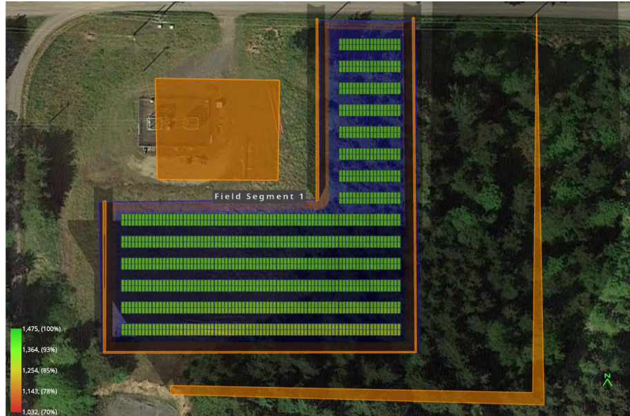
Figure 1.5. Shading Heat Map of PV Installation at Decatur Island Substation
