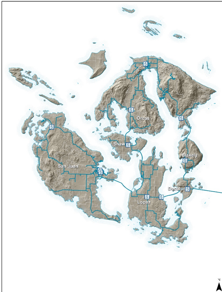
Figure 1.7. One Line Diagram of OPALCO's Transmission and Distribution System
