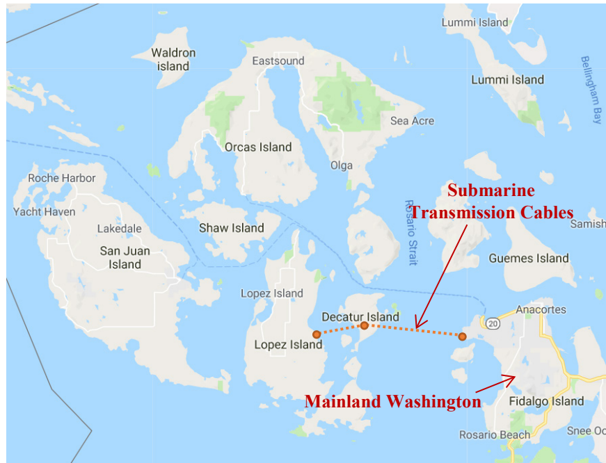
Figure 1.6. Transmission Cable Map from Fidalgo Substation in Anacortes to Decatur and Lopez Islands
